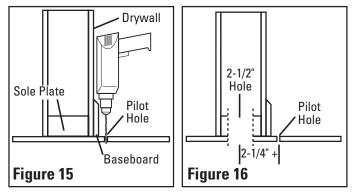
From below, locate the pilot hole and measure over approximately 2-1/4" (1/2" for the drywall + 1-3/4" to the center of a standard 2" x 4" sole plate). Add extra for any additional material such as baseboards, thicker drywall, etc. Using a 2-1/2" hole cutter, drill through flooring and sole plate. Using a flashlight, inspect the interior of the wall to confirm that there are no obstructions (Figure 16).
